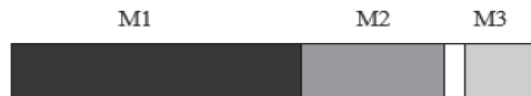
Figure 8 Gantt Chart with Expendability Space in M3 to be Given to M2
